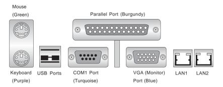
**Note:** COM2 is a header on the motherboard (see motherboard layout for location). The X5DLR-8G2+/X5DLR-8G2 does not have a parallel port.
